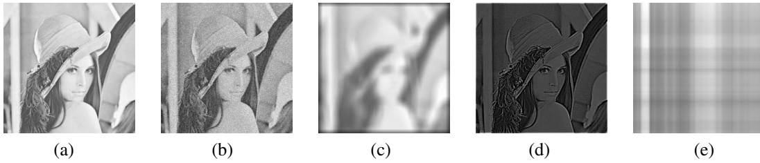
Fig. 2. (a) Original Image. Images constructed to have the same SSIM=0.50: (b) White Noise added, (c) blur distortion (d) high-boosted (e) Singular value decomposition (most significant eigenimage). Note that images with the same quality measure may have very different visual quality. The new index (QILV) seems to be more balanced.
