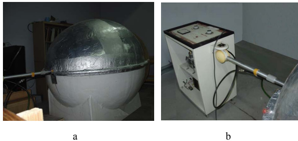
Fig. 1. a. Conductive wall cavity of Hyperthermia System b. Magnetron generator providing microwave energy of 200W at the frequency of 2450 MHz
