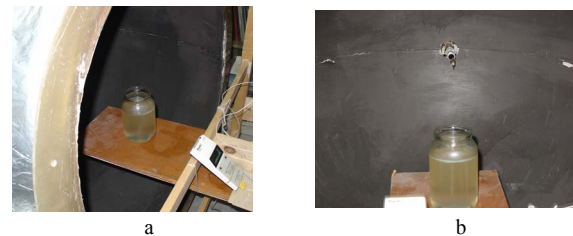
Fig. 9. a. Phantom placed on focal area and digital thermometer with measuring probe (side view) b. Ellipsoidal interior: phantom placed on focal area whereas dipole radiating antenna placed on second focus
