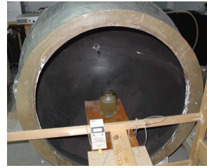
Fig. 2. Front view of the conductive wall cavity of the proposed Brain Hyperthermia System
