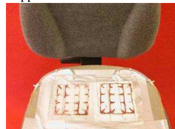
Figure 2: Flexible and active actimeter designed for a chair.
