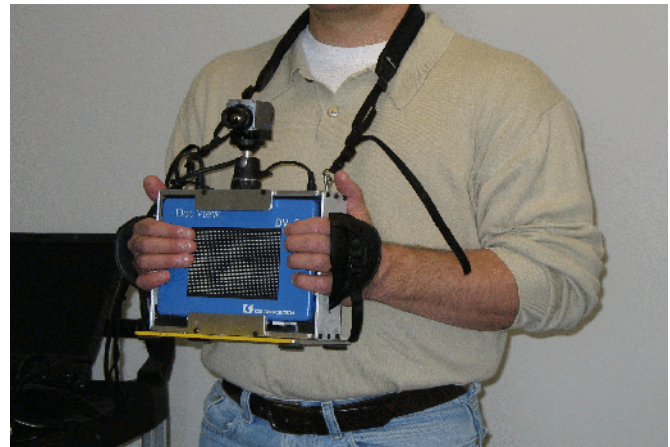
Fig. 1. Prototype device in hand held mode. The infrared camera is mounted on top of the tactile display. The tactile display shows the image of two people in front of the user.
