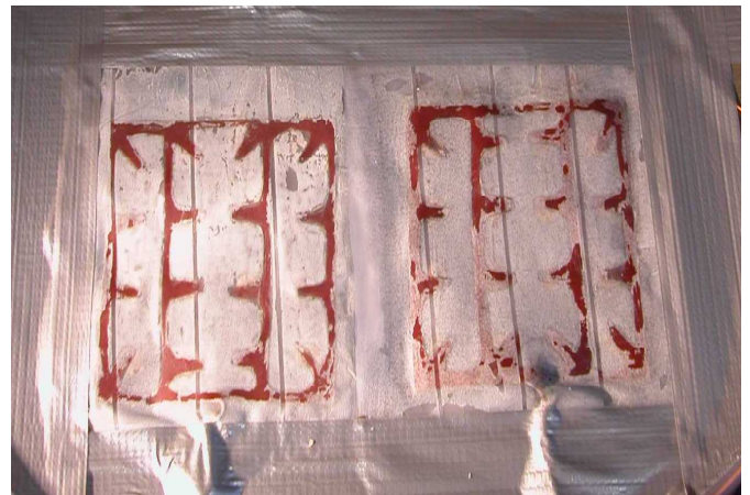
Fig. 1. View of the electropneumatic sensor. The 32 contacts are distributed in 2 groups
