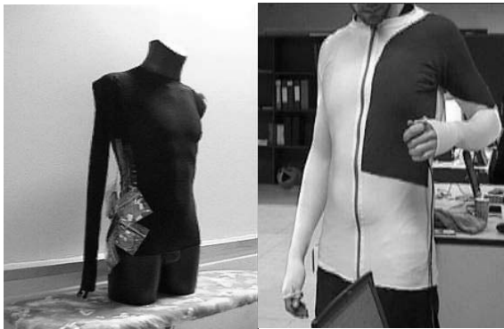
Fig. 8: Wearable interface to monitor movement and posture for post stroke rehabilitation: on the left handcraft prototype, on the right a prototype for industrial implementation.
