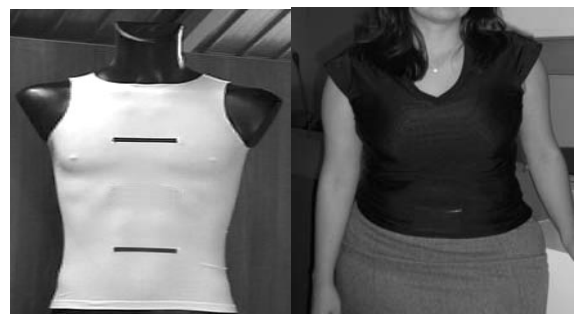
Fig. 6: Wearable interfaces: on the left a system to monitoring thorax and abdominal respiration signal; on the right the last generation of bio clothes, a female model.
