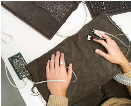
Fig. 9. Typical setup during hypoxia tests performed at CSEM. Two pulse oximeters and an altitude simulation mask were used to prove the ability of the finger ring to monitor oxygen desaturation at high altitudes
