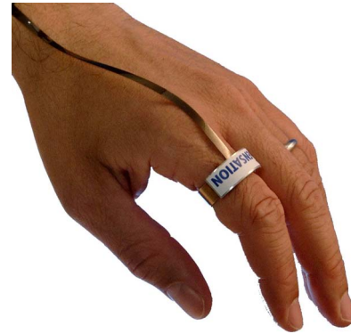
Fig. 1. The SpO 2 sensor integrated in a finger ring. The current prototype weights less than 5g and has demonstrated to be more comfortable than standard fingertip probes.
