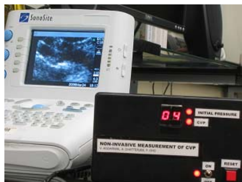
Fig. 4. Final CVP recording after IJ vein is fully collapsed.
