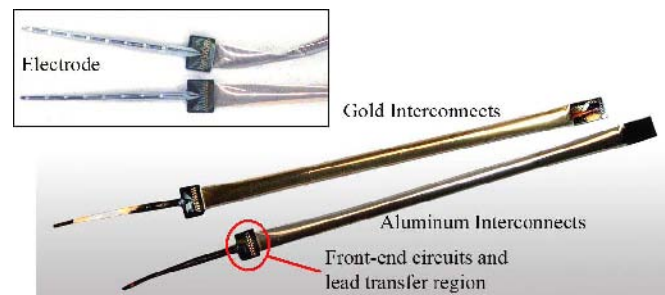
Fig. 11: A parylene-silicon electrode array (8mm) integrated with a cable (30mm) directly at the wafer level. In the future, front-end multiplexing and preamplification circuit will be integrated close to the electrode, improving noise immunity and minimizing the number of the leads transferred.
