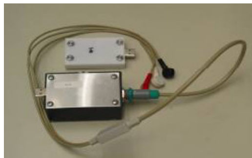
Fig. 3. A single transmission mote and a single receiver mote for wireless ECG data collection.
