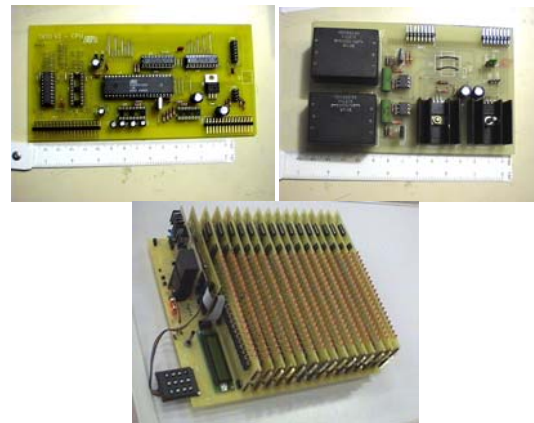
Fig. 3. CPU, power supply and stimulation boards of the second prototype
