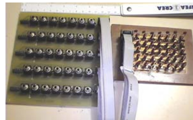
Fig.8. The RMS current measurement board and skin simulator board
