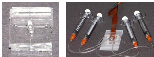
Fig. 3. Photograph of the assembled two layer structure with wells, ports and interconnects formed (left) and the complete micro-incubator (right).
