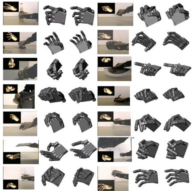
Fig. 7 pictures of data capture using cyber glove, robotic hand posture created with actuator without grouping of the actuators, and robotic hand posture created with just 6 clusters. 14 different hand postures are used.
