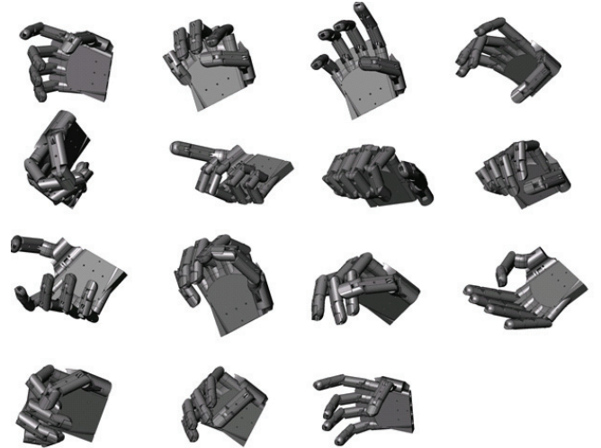
Fig. 3 Fifteen robotic hand postures used in the design. Joint angles for each posture are captured using the cyber glove and transformed into joint angles for the robotic hand.
