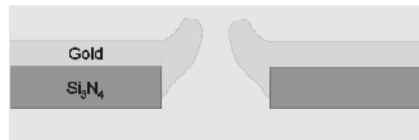
Fig. 2. Cross section schematic of the customized Nanopore. Biological macromolecules can be attached on the gold.
