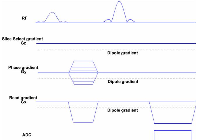
Fig. 3. Spin echo sequence used for imaging magnetic equipotentials.
