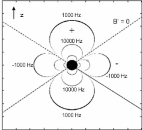
Fig. 1. MATLAB Simulation of the spatial distributions of the resonant frequency.
