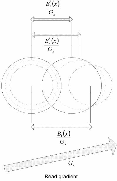
Fig. 4. Schematic view of the effect of the background gradient on the geometric encoding errors.
