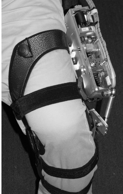
Fig. 6. Photo of the prototype FlexCVA attached to a knee brace. Future versions will reduce the size and allow the entire device to fit under loose-fitting clothing.
