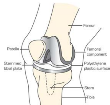
Fig. 1. Components in total knee replacement prosthesis. Components replace diseased joint surfaces.
