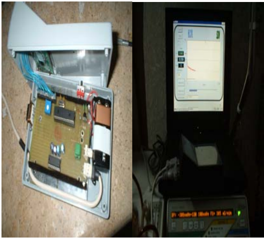
Figure 1: Experimental Prototype by using PIC Micro controller and connection in arterial line the Hemodialysis machine.
