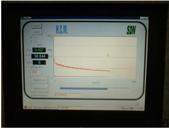
Figure 3: Evolution of the urea concentration estimated from the optical transmittance during the experimental Hemodialysis procedure in a patient.
