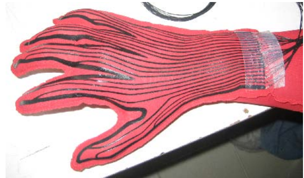
Fig. 1. The Sensing Glove realized by CE sensors directly integrated in the fabric. Twenty sensors ( S_1-S_{20} ) are distributed over the hand.
