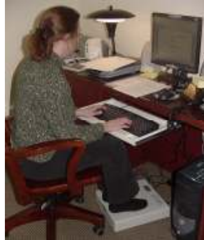
Figure 2: Plantar stimulation device utilized in the seated position. A resonance based design allows a small electromagnetic actuator to provide the 50 \mu\text{m} displacement to the plantar surface of subjects. The lack of any direct attachment to the patient allows convenient use.
