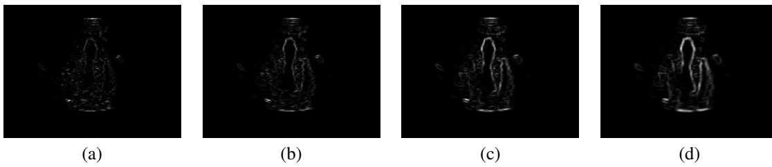
Figure 3. Effect of window size. From left to right: 3x3, 5x5, 7x7, 9x9.
