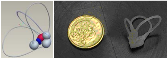
Fig 7. The vestibular system CAD model (left): the three semicircular canals are in light color and the two otolithic organs, sacule and utricle, in dark. The microfabricated vestibular system compared with a 10 eurocent coin (right).
