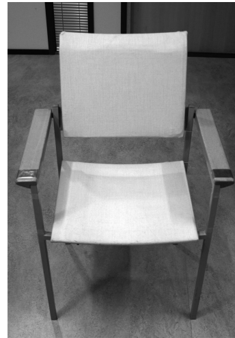
Fig. 1. The wireless EMFi-BCG measurement chair. The electronics are hidden under the chair. EMFi sensor films are fitted under the upholstery on the seat and the back panels of the chair. Small copper strips have been fitted to the armrests to measure the ECG.
