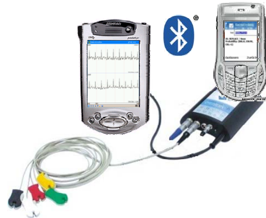
Fig. 2: Mobile pacemaker follow-up unit. ECG signals are recorded with a mobile biosignal acquisition system (g.mobilab, g.tec – Guger Technologies OEG) that is connected with a PDA. A mobile phone is used for transmitting the ECGs to the telemedicine service centre over the UMTS network.
