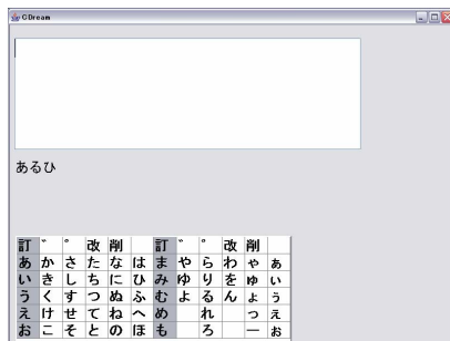
Fig. 5. An execution screen of the scanning communication system.
