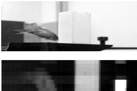
Fig. 13. Acquired image from the polycrystalline CZT
