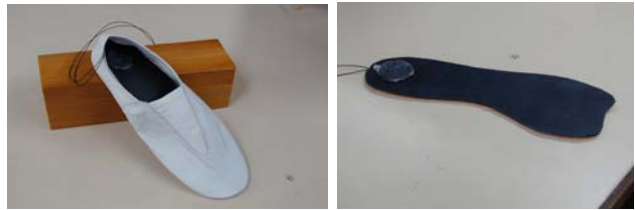
Fig. 1. Sensorized shoe for marking the gait cycle.
