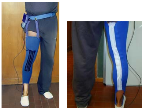
Fig. 3. The overall prototype consisting of a KB, sensorized shoe and an “on body unit”. Front (left side) and back (right side) views.
