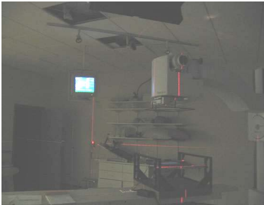
Fig. 1. Alignment of the lasers on the reference frame.
