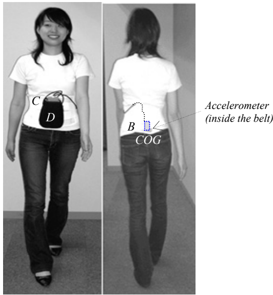
Fig. 1b. The COG of young subject was measured by a portable measurement system using accelerometer while walking.
