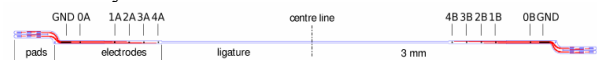
Figure 4 Scheme of a tf-LIFE electrode. Total length:60 mm, pad area length: 5mm. GND is a ground electrode and (L1-L4, R1-R4) represent the recording sites.
