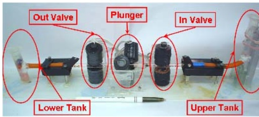
Figure 4. The experimental prototype used in this work. The valve two coil in the left realize the valve while the three coil in the right realize the plunger.
