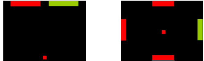
Fig.1. Left and right panels are representative of 1-dimensional and 2-dimensional tasks used on-line to test the applicability of linear inverse procedure. In the left panel red cursor move upward at a fixed rate while the user control horizontal movements (towards green targets). In the right panel the cursor is controlled completely by the user.
