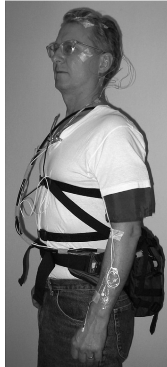
Fig. 3. Data collection setup with EEG, EOG, EKG, twin respiration, skin temperature, electrodermal sensors, and blood pressure cuff.
