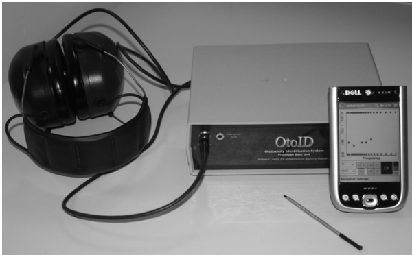
Fig. 8. New mobile ototoxicity monitoring system with audiometric base unit shown in center and headphones shown at left. The PDA device runs the monitoring application software.
