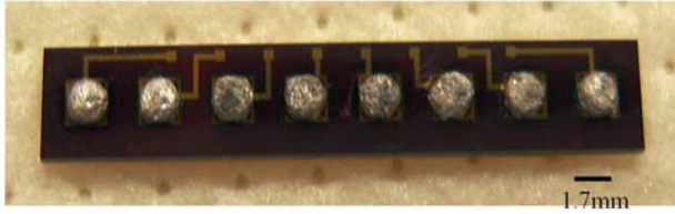
FIGURE 5. A photograph of an 8-element transducer array
