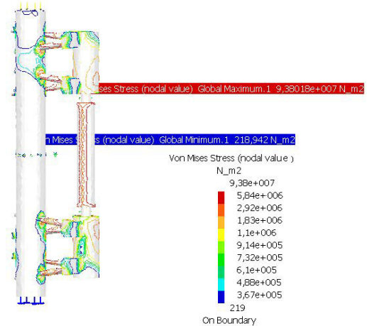
Fig. 4. Stress distribution at the beginning of the fracture healing process (granulation tissue at fracture gap). Load -150N, 1mm transverse fracture gap, 60 mm distance between bone and fixator's frame
