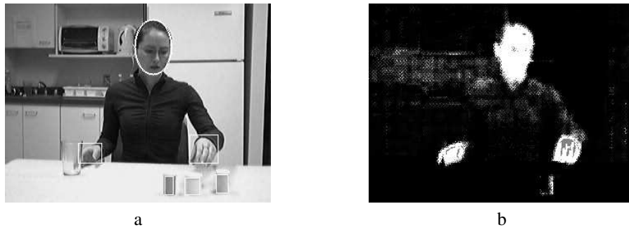
Fig. 1. a) Mobile objects detection and tracking and b) corresponding skin color likelihood map.
