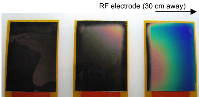
Figure 9. Representative image of groundpad heating when pads are activated simultaneously. The proximal pad (right) heats up most with little heating of the other pads. Temperature sensitive LCD paper shows pad surface temperature profile (red = 25°C, blue = 30°C).
