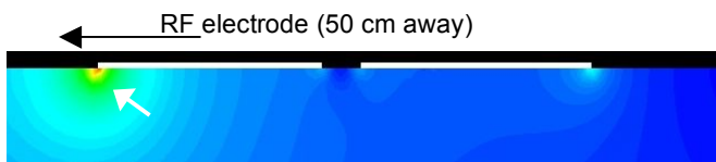
Figure 3. RF current density in a computer simulation. Current flows preferentially to the leading edge of the closest pad (white arrow).
